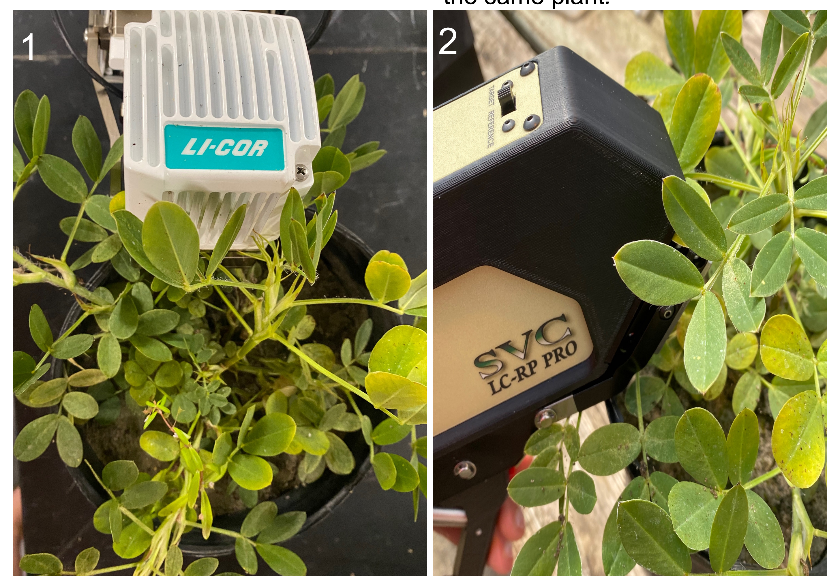
Figure 3. A suite of physiological measurements which will be taken throughout the course of the peanut's life cycle. These will include gas exchange (1), hyperspectral reflectance (2), relative water content, leaf water potentials and chlorophyll fluorescence (not shown)
